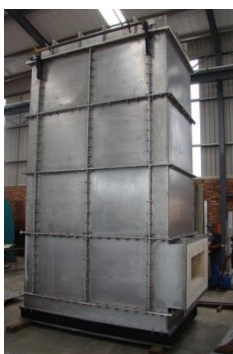
Adsorb APF100 is a pyrolysis-combustion hybrid designed to process primarily biomass residues
