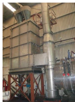
Adsorb APF100 is a pyrolysis-combustion hybrid designed to process primarily biomass residues
